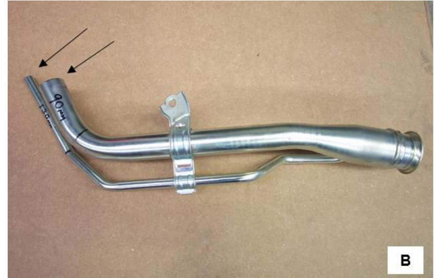
PICTURES A & B Filler Neck - Measure 90mm from the centre of the bend and cut Fast Fill Vent - Measure 130mm from the bend and cut.
