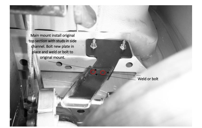
Use this section and weld to new plate provided for rear mount behind muffler. See Item 2
