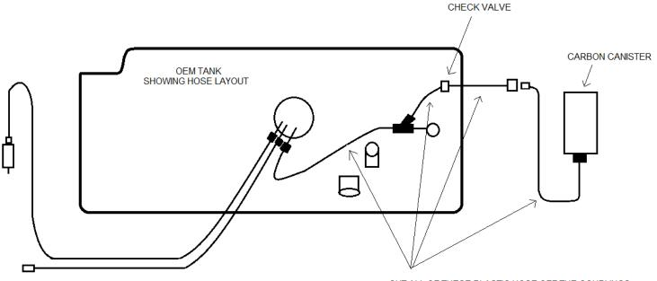
CUT ALL OF THESE PLASTIC HOSE OFF THE COUPLINGS AND RETAIN THE COUPLINGS, Y PIECE AND CHECK VALVE
