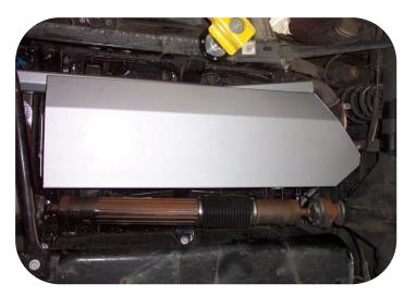
All auxiliary tanks come complete with a quality LED Switch Gauge unit which shows the fuel level in the auxiliary tank and incorporates the switch to
