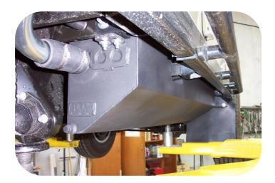
All auxiliary tanks come complete with a quality LED Switch Gauge unit which shows the fuel level in the auxiliary tank and incorporates the switch to operate the transfer pump.
