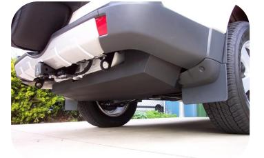
auxiliary tanks come complete with a quality LED Switch Gauge unit which shows the fuel level in the auxiliary tank and incorporates the switch to operate the transfer pump.
